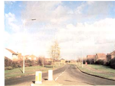
The main route into a new neighbourhood. Everyone accesses along it, yet the houses turn their backs onto it. The result is a soulless place where pedestrians feel insecure and where drivers are 'encouraged' to drive fast. (p.11)
