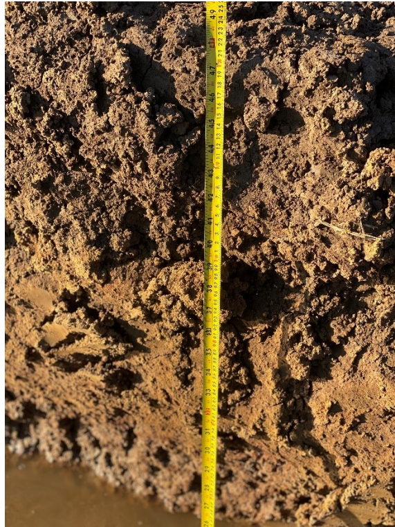
Image 2- Soil Pit 3. Clearly showing the different silty clay loam horizons, slowly permeable layers and therefore imperfect drainage ability indicating wetness as a trigger for ALC grading.
